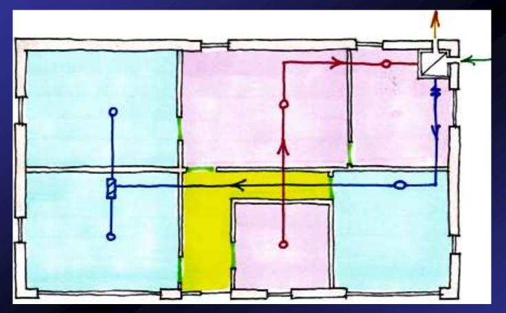
The design of the system must be balanced for the entire dwelling to ensure that a minimum air change rate of 0.3 changes per hour is achieved.
