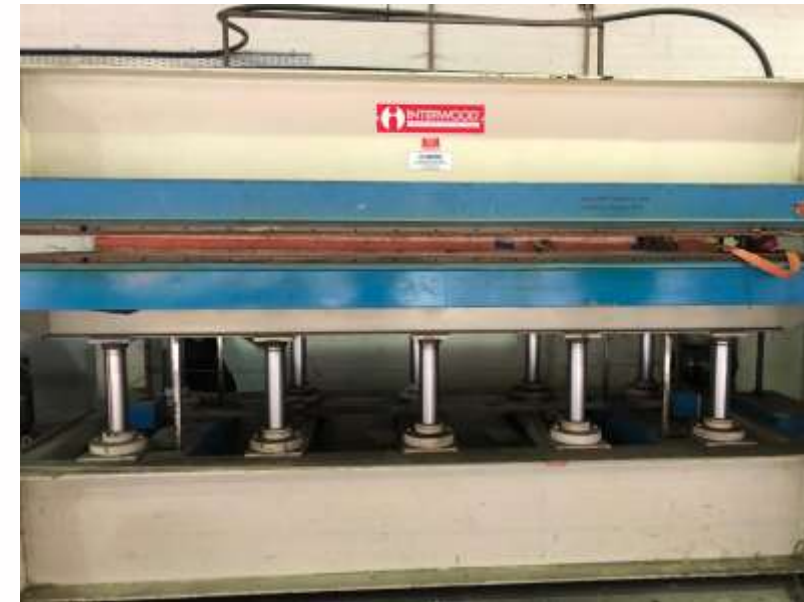
CLT panel subjected to pressure
