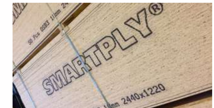
Panel products (Orientated strand Board, Plywood, MDF) e.g. flooring, wall sheathing, facades
